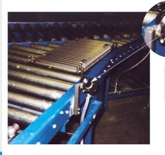
**DRYING ENAMEL BASED PAINTS** Side mounted AM40 airmover drying enamel paint on a radiator manufacturing line.
