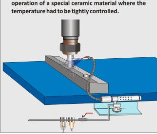
A Model 57025AS is used to cool a milling
